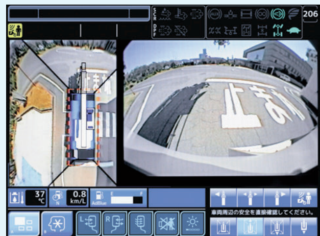
The large monitor gives an all-round bird's-eye view from above and shows any vulnerable road users approaching alongside
