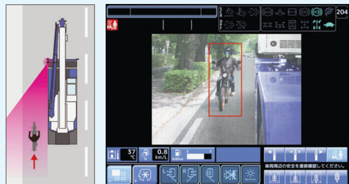
The large monitor gives an all-round bird's-eye view from above and shows any vulnerable road users approaching alongside
