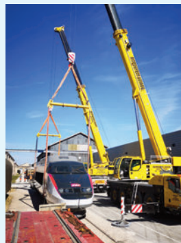
Above: The two Tadano Demag cranes work together to lift the 34-tonne train
