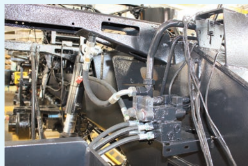
Blasted and primed with zinc dust
