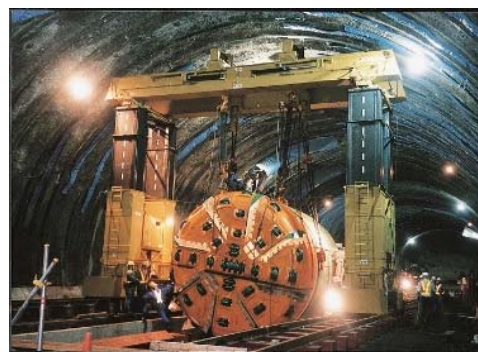
Hydraulic gate-shaped lifters : TB-1000
