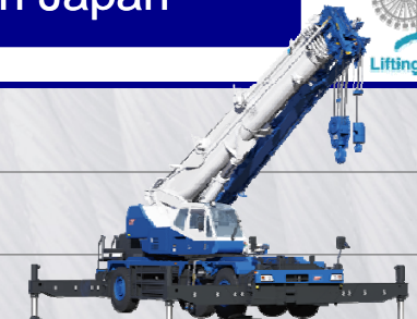
A promising new three-axle 50t Rough Terrain Crane equipped with 3-staged jib, boasting the highest lifting height of its class GR-500N: Released in April 2015
