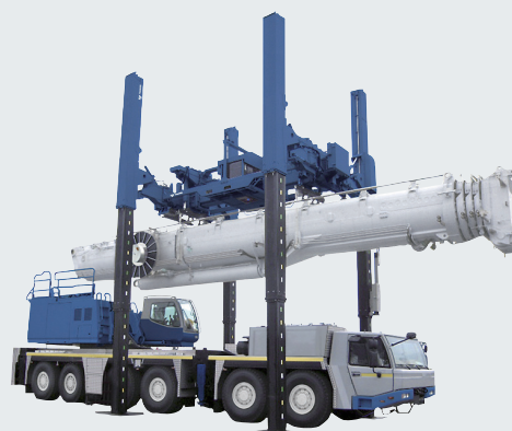
All Terrain Crane Mounting/Removal Lifter (Example of boom removal from ATF400G-6)
