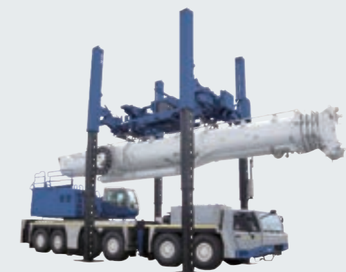
All Terrain Crane Mounting/Removal Lifter (Example of boom removal from ATF400G-6)
