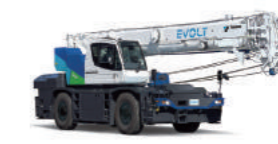
Electric rough terrain crane GR-250N EVOLT
